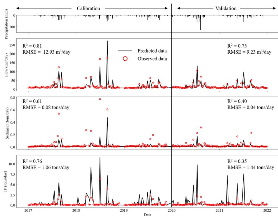
**Figure 4.** Results of calibration and validation of the SWAT model.
