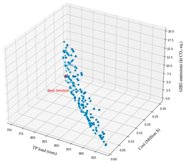
Figure 6. Multi-objective optimization results using NSGA-III (3D).
