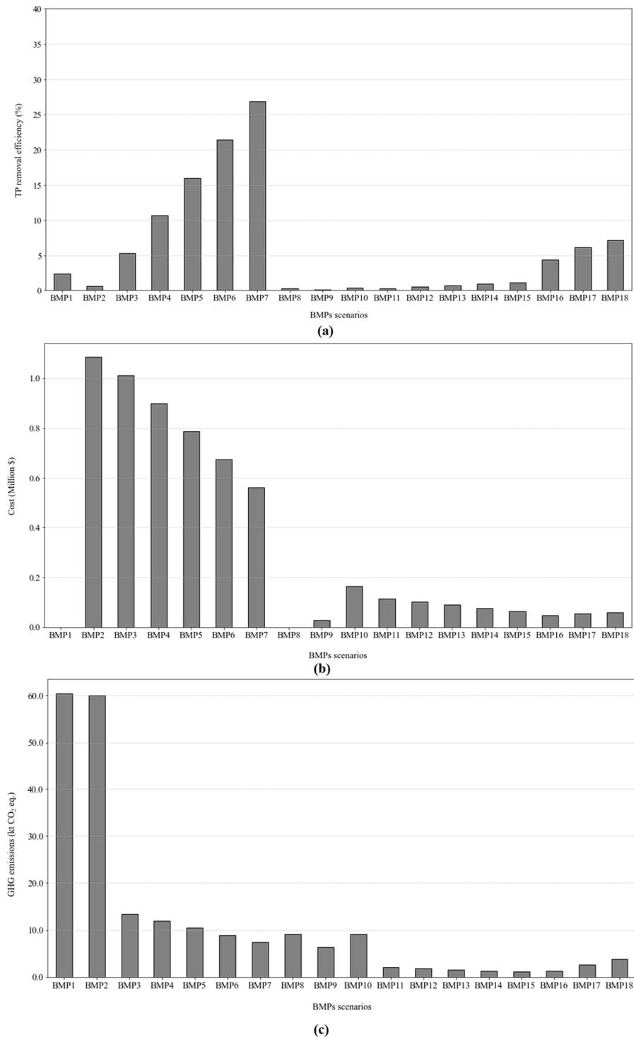
**Figure 5.** Comparative analysis of TP removal efficiency, cost, and GHG emissions when applying individual BMP scenarios: (a) expected TP removal efficiencies, (b) expected cost, (c) expected GHG emissions when applying individual BMP scenarios.
