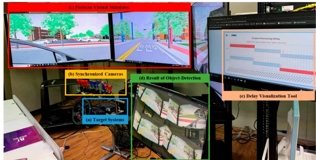
**Figure 10.** Prototype of the delay measurement environment with H/W and S/W.
