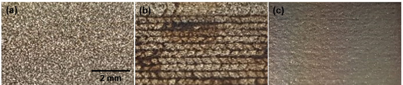
Fig. 2. Surface photographs of the untreated (a), LSP-treated (b) and UNSM-treated (c) samples.
