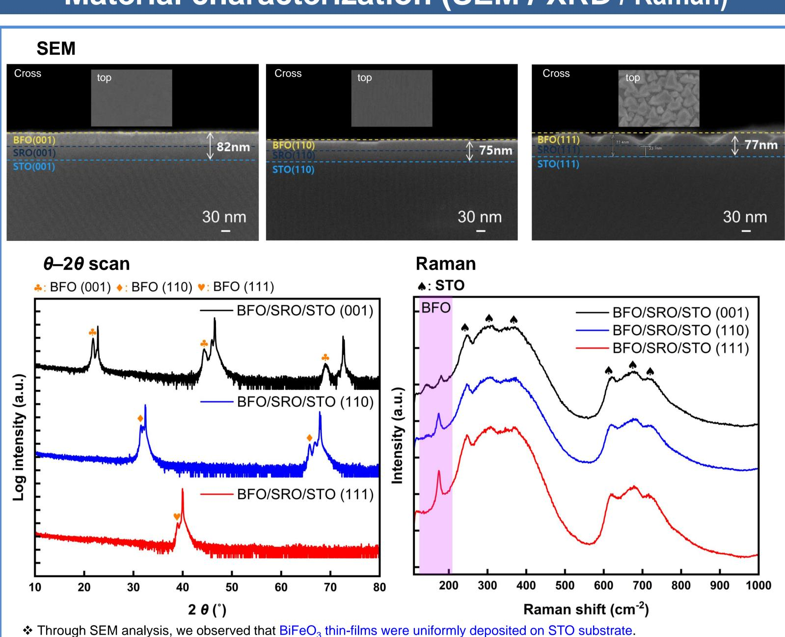
In order to confirm the crystallinity of the prepared sample, XRD and Raman analyzes were performed, and as a result, the characteristics of a single crystal thin film were shown according to the crystal orientation.
