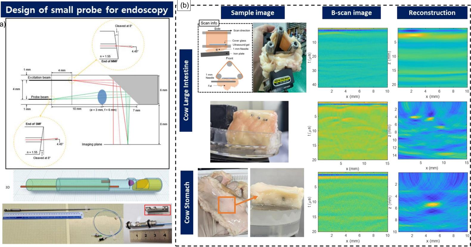
(a) Design the probe outer diameter 7 mm, inner diameter 6 mm
