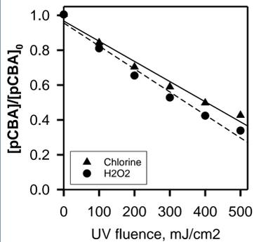
❖ The degradation rates of pCBA during UV/Chlorine and UV/H<sub>2</sub>O<sub>2</sub> were comparable as a function of UV fluence in the tested oxidant conditions (4 ppm Cl<sub>2</sub> and 5 ppm H<sub>2</sub>O<sub>2</sub>).
