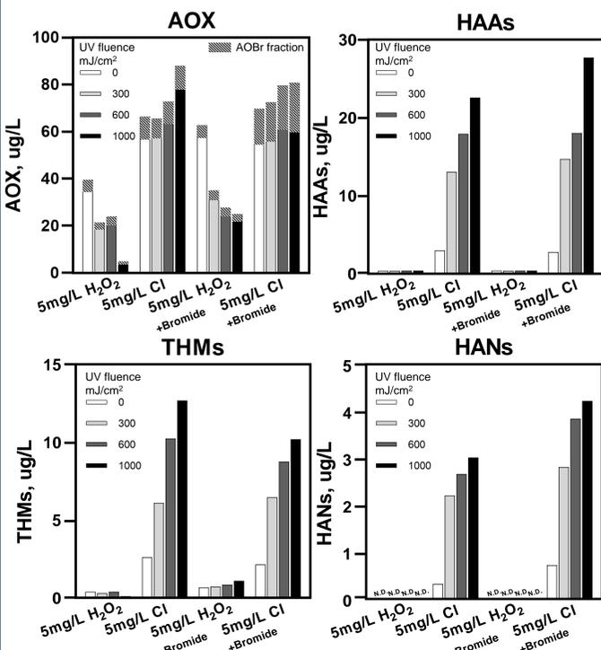
Figure 2. Formation of DBPs during treatment of 5mg/L H<sub>2</sub>O<sub>2</sub> or chlorine, coupled with 0–1000 mJ/cm<sup>2</sup> UV dose with and without 100ppb bromide spiking
