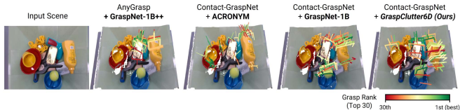
Fig. 9. Grasp predictions (top 30) in a real-world pile scene.
