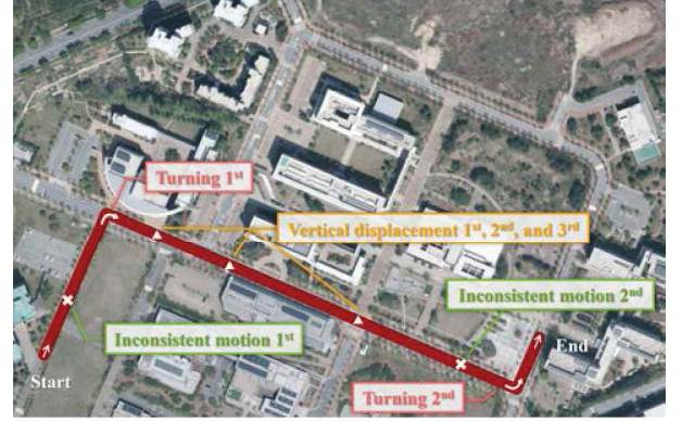
Figure 3: Experimental route, covering 600 m with an average vehicle speed of 20 km/h
