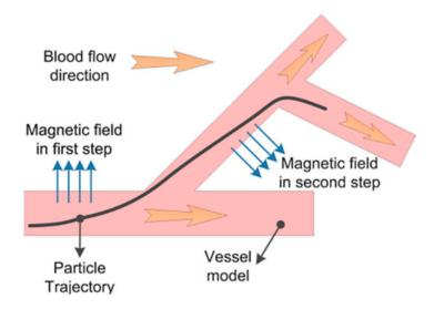
Figure 1. Guidance scheme of magnetic nanoparticles at blood vessel by applying magnetic force.
