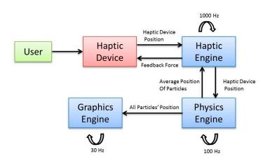
Figure 4. System architecture and data flow of different modules.
