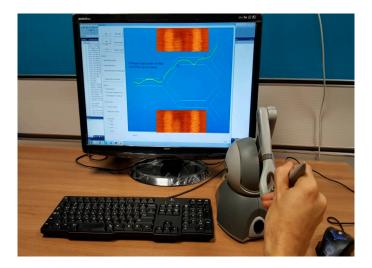
Figure 2. Virtual tele-nano-manipulation system.
