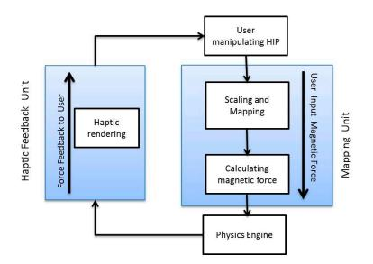
Figure 5. Haptic engine unit for tele-manipulation of magnetic nanoparticles (MNPs).
