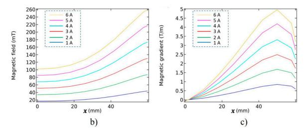
**Figure 7.** Electromagnetic actuation system applied to the developed virtual reality (VR) simulator. (a) Electromagnetic nano actuation system setup and its different parameters (all the dimensions are in mm). (b,c) Spatial distribution of the magnetic field and magnetic gradient in practice, respectively; when current from 1 A to 6 A is applied to the right coil. We used the Bell-5180 Gaussmeter (Transcat, Inc., Rochester, NY, USA) to record this data.
