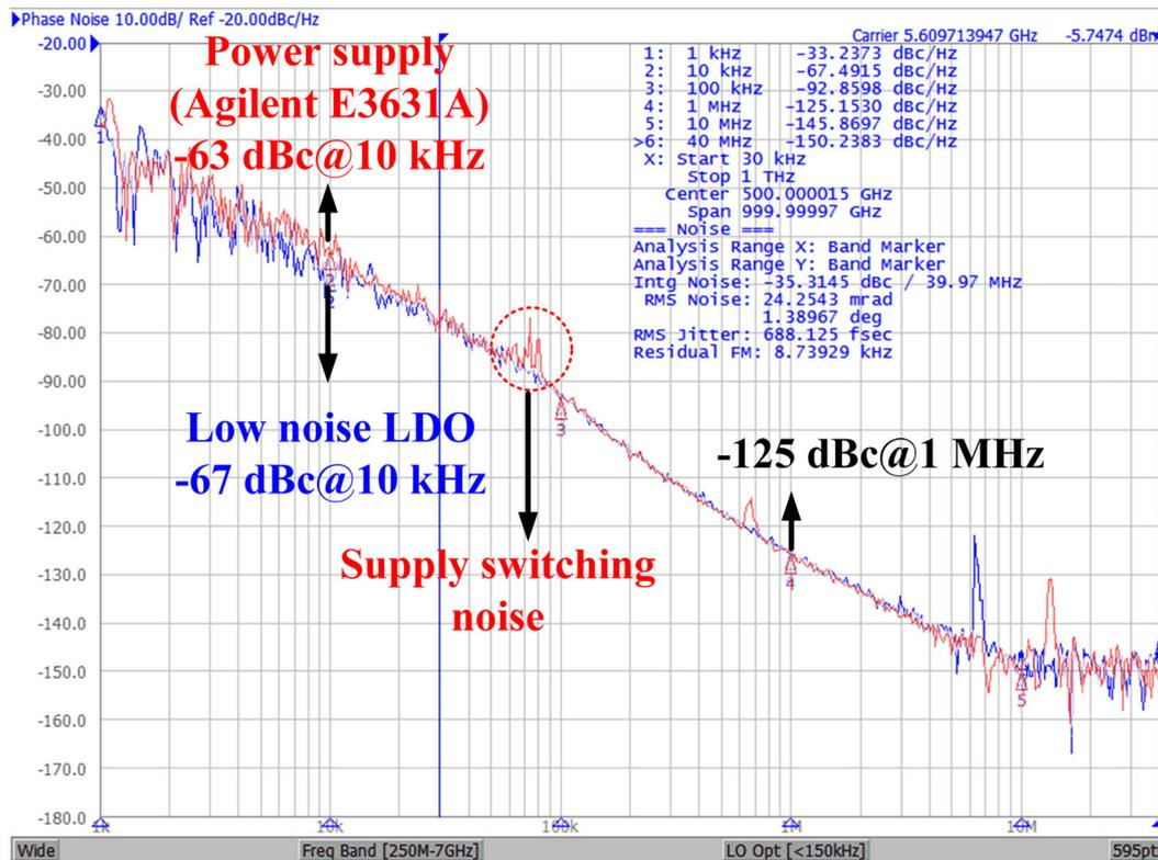
FIGURE 17 Comparison of voltage-controlled oscillator (VCO) phase noise with low-noise low drop-out (LDO) [Colour figure can be viewed at wileyonlinelibrary.com]
