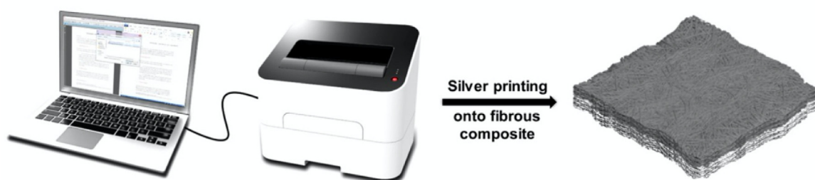
Fig. 9. The steps of the silver nanoparticle printing process on electrospun membrane. The image is reproduced from a previous study [99] with the permission of Elsevier.
