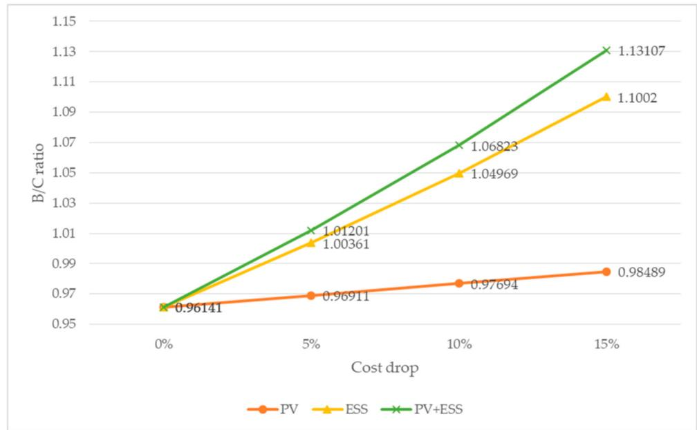
Figure 8. B/C changes owing to the equipment cost drop.
