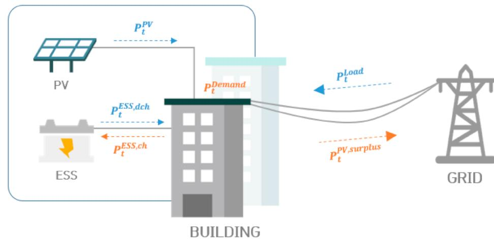
**Figure 2.** DER structural diagram for buildings considered in this study.
