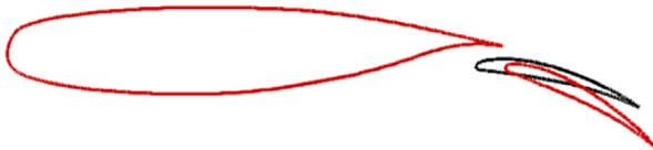
**Fig. 10.** Comparison of baseline and design results in geometry — Black : Baseline, Red : Optimum. (For interpretation of the references to color in this figure legend, the reader is referred to the web version of this article.)
