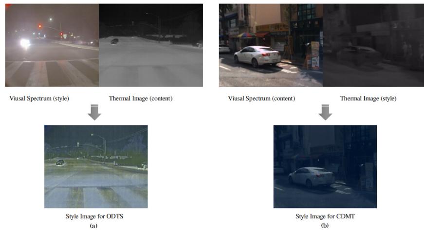
Fig. 1. (a) Object detection in thermal images through style consistency (ODSC). Visible spectrum (RGB image) is treated as a style image whereas, the thermal image is considered as content image. The output shows the enhanced image having low-level features adapt from the visible spectrum. (b) Cross-domain model transfer with style transfer. Style from the thermal image is transferred to the visible spectrum (RGB content image).
