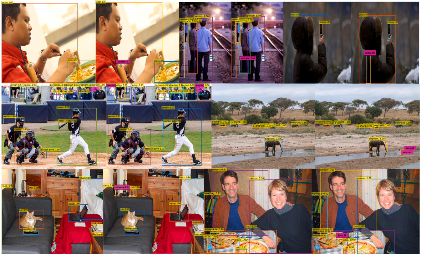
Fig. 7. Qualitative analysis of SOF-DETR, where we have several pairs of images with the first and second images illustrating detections from DETR and SOF-DETR, respectively. Additional detections through SOF-DETR are represented with a pink color class box. Detections only with more than 90% confidence value are displayed.
